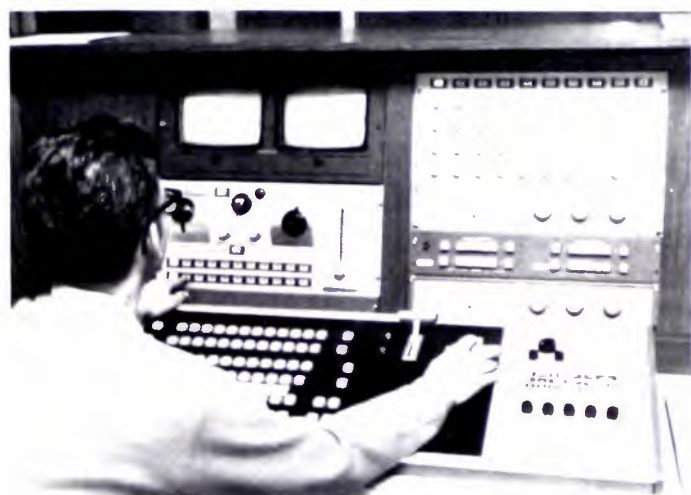
Power Optics' remote control panels installed on WJLS's main control console (facing camera bottom left and top right).
